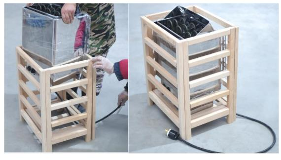
7. Install the vertical bench by inserting it into the channels on the side walls. Set the horizontal bench on top of the vertical bench and secure it with screws.
