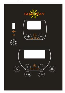
1.Power button , to turn on/off the power to the cabin.
